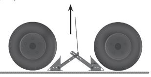
9) To lock the chock, step the chock into place tightly between the wheels. Place the padlock through one of the empty holes in the center of the arms, or through one of the lock holes in the wedges just above the scissor arms. Note: The lock is to be used as a theft deterrent. The lock will not guarantee the chocks can not be stolen.
