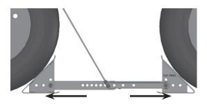
3) Slide the clevis pin into one of the holes in the arms to temporarily hold them in place. Don't insert the cotter pin yet.
