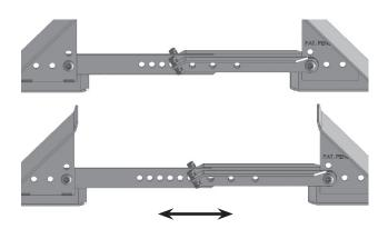
5) Place the clevis pin into one of the sets of holes, and then replace the cotter pin to secure it.
