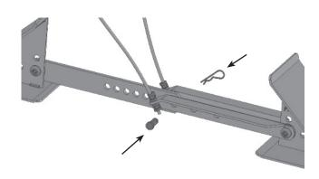
If you are not able to lengthen or shorten the chock to fit your axle spacing using the arm holes for adjustment, the bolts holding the ends of the scissor arms can be moved. Use the included hex key (Allen wrench) and a socket wrench to move the bolts to either of the other two adjustment holes in the wedges.
