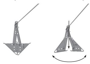
6) Slide the chocks into position between the tires so that the wedges are centered on the tread of the tire. Step down on the center of the arms to force them out against the tires and lock them into place.
