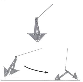
Others prefer to place the pin so that the arms hang at about the same length, and then step down on the tail ends of the wedges to force them open before sliding them between the wheels. Try each way a few times to see which works best for you.
