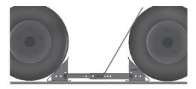
8) To remove the chocks, grasp the handle firmly in the middle and pull upward.
